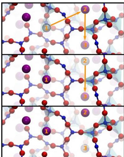
Figure 1: Visualization of the diffusion model by a series of snapshots: large magenta spheres are  $\text{Rb}^+$  ions, white spheres vacancies, small red circles oxygen and blue are boron atoms. From top to bottom: vacancy makes successive jumps on the three-dimensional arrangement of  $\text{Rb}^+$  ions.
