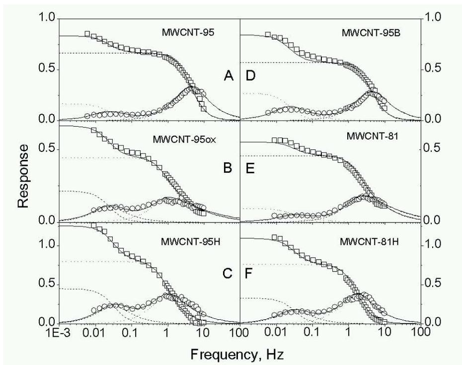
Fig. 3. FR sorption rate spectra for the sorption of cyclopropane, recorded at 0 °C and 133 Pa using 200 mg of <150- μm size particles. Sample MWCNT-81 was obtained from MWCNT-95B by oxidative treatment. The MWCNT-81H was prepared from the MWCNT-81 by thermal treatment at 900 °C in argon. The same procedure was applied with the carbon nanotubes having the original length.
