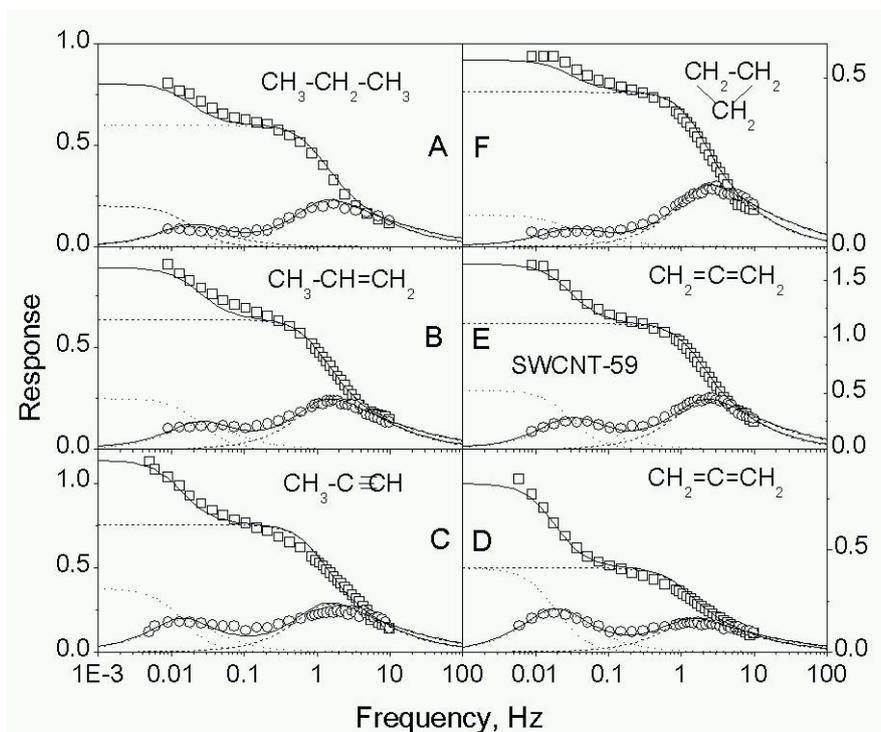
Fig. 4. FR rate spectra for the sorption of various  $C_3$  hydrocarbons, recorded at  $0^\circ C$  and 133 Pa using 200 mg of  $<150\text{-}\mu m$  size particles on sample MWCNT-81 and SWCNT-59.
