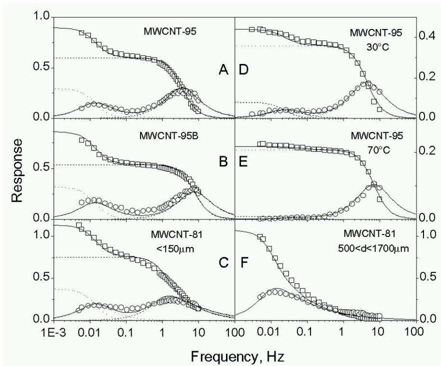
Fig. 2. FR spectra of propyne sorption on MWCNTs at 0 °C and 133 Pa. Each measurement was made on 200 mg CNT. Symbols correspond to the in-phase ( $\square$ ) and out-of-phase ( $\circ$ ) components of the experimentally determined response functions. Full lines are the best-fit characteristic functions.
