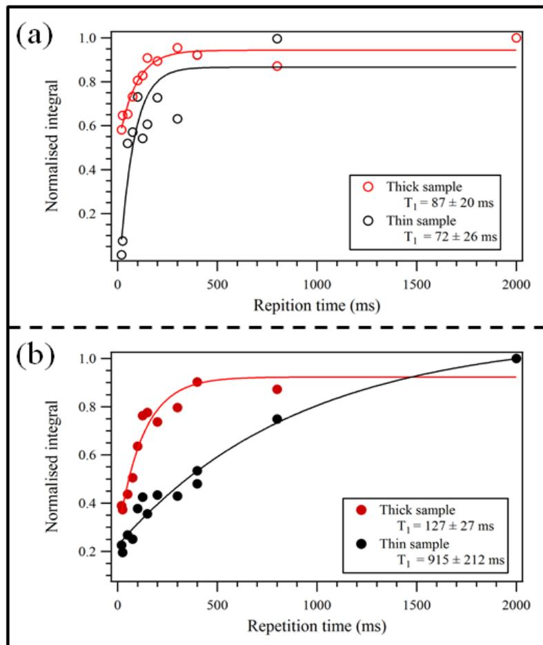
**Fig. 4:**  $T_1$  measurement taken using multiple CPMG sequence with different repetition times; 2048 scans on the two different samples. (a) Bar magnet style sensor, 16 echoes summed,  $\tau_E = 50 \mu\text{s}$ . (b) Four magnet surface sensor, 64 echoes summed,  $\tau_E = 100 \mu\text{s}$ .  $T_1$  values were extracted from the fittings, they are displayed along with their associated fitting parameter errors.
