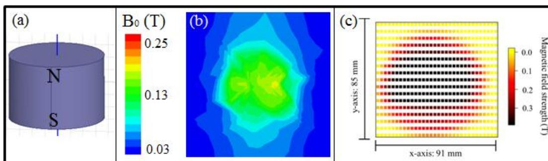
**Fig. 2:** (a) Schematic of the bar-magnet unilateral surface sensor. A uniform magnetic field is generated above the magnet. A single-turn butterfly coil is used for RF transmission and receiving. (b) A computer simulation of the magnetic field over the surface of the magnet. The colour bar is to help illustrate the field homogeneity, and does not represent true magnetic field values. (c) A magnetic field map for the field 5 mm above the magnet surface.
