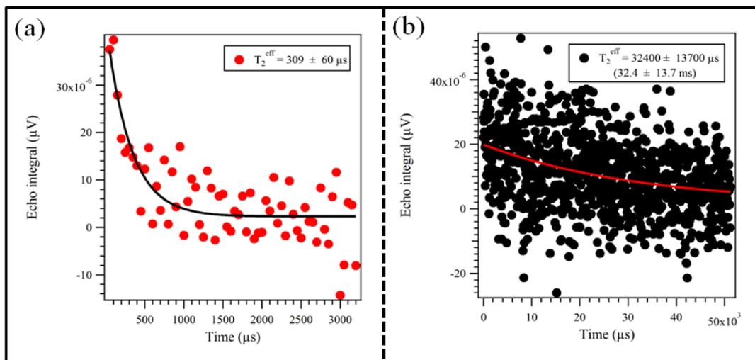
**Fig. 3:**  $T_2^{\text{eff}}$  measurement taken using a CPMG sequence;  $\tau_E = 50 \mu\text{s}$ , 2048 scans on the thin sample. (a) Bar magnet style sensor, 64 echoes. (b) Four magnet surface sensor, 1024 echoes.  $T_2^{\text{eff}}$  values were extracted from the fittings, they are displayed along with their associated fitting parameter errors.
