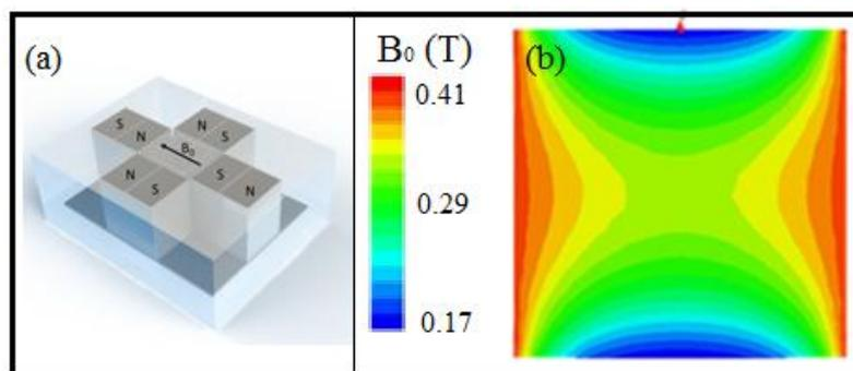
**Fig. 1:** (a) Schematic of the four magnet unilateral surface sensor. A uniform magnetic field is generated in the magnet gap. A two-turn surface coil is used for RF transmission and receiving. (b) A computer simulation of the magnetic field over the surface of the magnets. The colour bar is to help illustrate the field homogeneity, and does not represent true magnetic field values.
