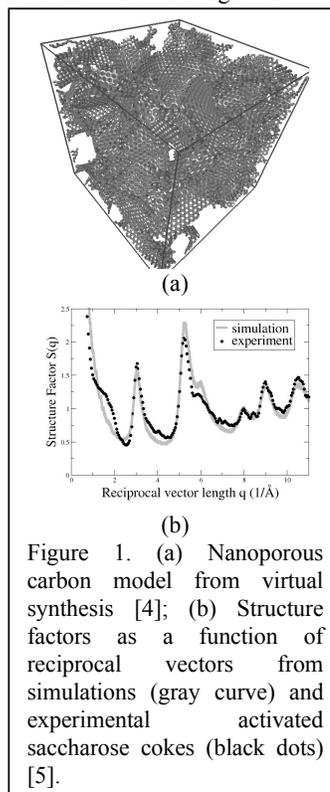
Figure 1. (a) Nanoporous carbon model from virtual synthesis [4]; (b) Structure factors as a function of reciprocal vectors from simulations (gray curve) and experimental activated saccharose cokes (black dots) [5].
