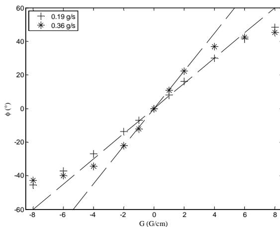
**Fig. 4:** Mean phase shift ( $^\circ$ ) according to the strength of gradient (G/cm) for velocity measurements in a packed bed of polystyrene beads (0.5 mm in diameter) and with a 20 mm slice selection. The dotted lines represent the linearization of the curves near the origin. The flow rates are respectively 0.19 g/s and 0.31 g/s.
