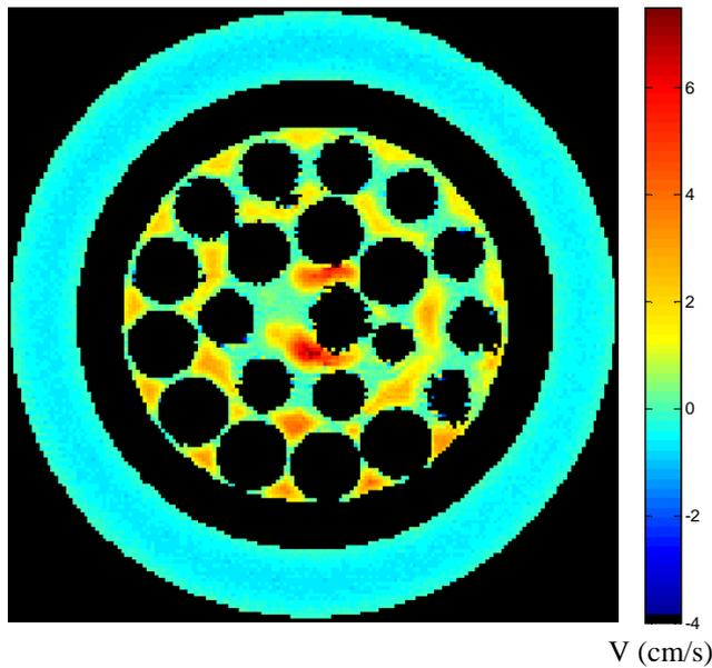
**Fig. 2:** Velocity map obtained by MRI velocimetry with a 1 mm thickness for slice selection. Areas in black correspond to the absence of signal (solid). The porous part contains a packed bed of polyacetal beads (3.175 mm in diameter). The mass flow rate is equal to 0.914 g/s.
