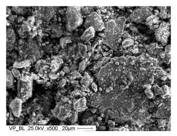
Fig. 1 Scanning electron micrograph of BFS particles.
