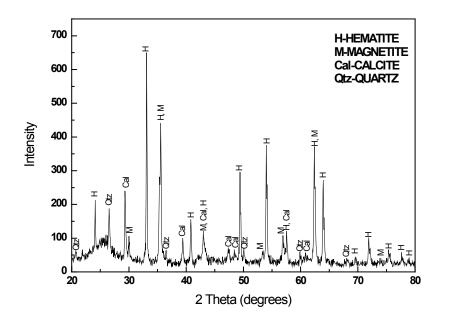
Fig. 3 X-ray diffraction pattern of the BFS sample.
