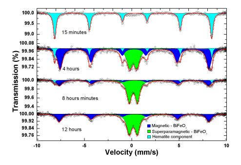
Fig. 2 Mössbauer spectra of BiFeO<sub>3</sub> prepared by ball milling of the Bi<sub>2</sub>O<sub>3</sub>/Fe<sub>2</sub>O<sub>3</sub> mixture for: 15 min, 4 h, 8 h and 12 h.
