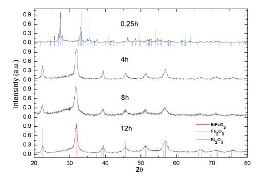
Fig. 1 X-ray diffraction of  $Fe_2O_3/Bi_2O_3$  milled for: 0.25 h, 4 h, 8 h and 12 h.
