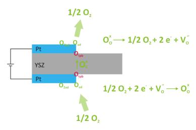
**Fig. 1** The oxygen exchange processes at the tpb during electrochemical polarization.
