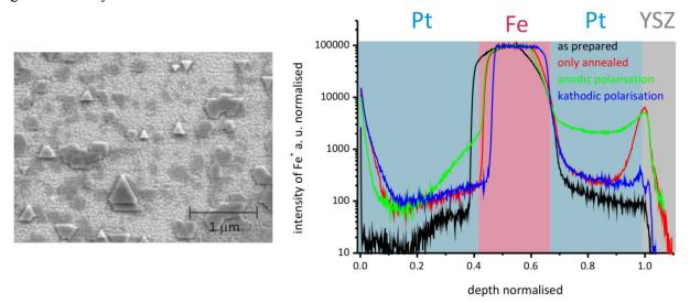
Fig. 3 Left: SEM picture of a sample annealed in air showing iron oxide islands. Right: SIMS depth profiles of different pieces of a sample exposed to different conditions.
