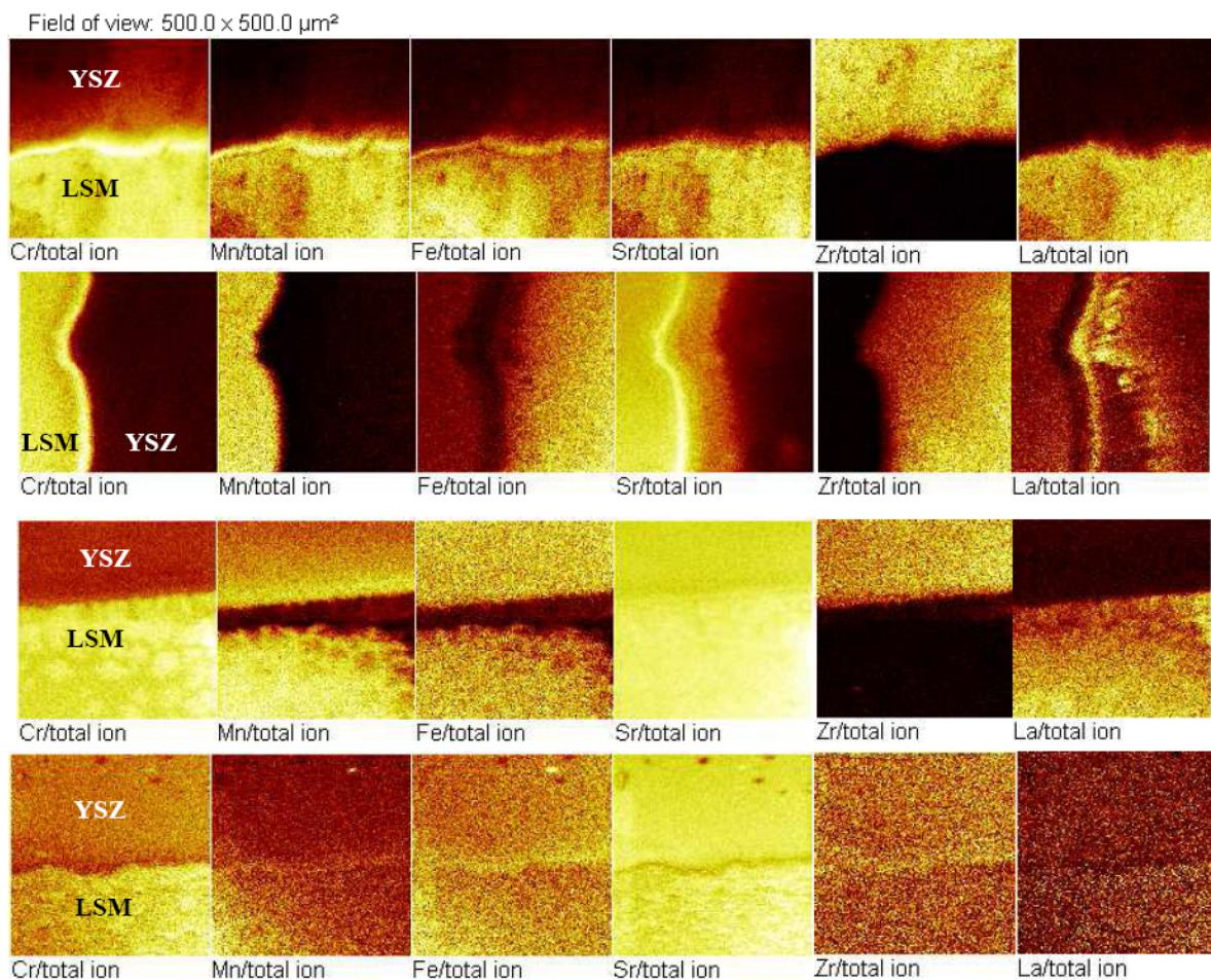
**Fig. 1** ToF-SIMS images of an LSM electrode on a YSZ sample. The whole sample was split into four smaller samples. Each quarter was annealed for different times at 1000 °C. The first line shows the sample as prepared without annealing. The other lines show the annealed quarters after 10 hours, 30 hours and 100 hours. Electrochemical polarization was not performed [3].
