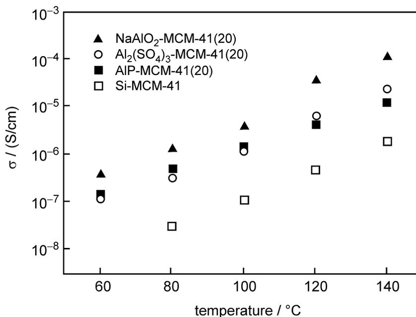
**Fig. 1** Proton conductivities at 100% relative humidity of mesoporous MCM-41 materials with a Si/Al ratio of 20 compared to pristine Si-MCM-41.
