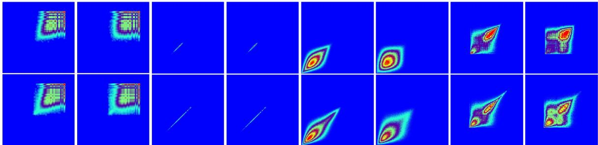
**Fig. 2:** Exchange plots for NZ sand (*top*) and Mt. Gambier limestone (*bottom*), with  $t_E = 100ms$  in pairs of two exchange times  $t_D = \{3;300\}$  ms. From left to right:  $T_2$ - $T_2$  from NMR simulation,  $d_{vs}$ -  $d_{vs}$ ,  $d_{EDM}$ - $d_{EDM}$ ,  $T_{2CDM}$ - $T_{2CDM}$ . Axes are logarithmic (pairs from left to right) in [3;300]ms, [3.36;1680] $\mu m$ , [3.36;1680] $\mu m$ , [0.01;10]s.
