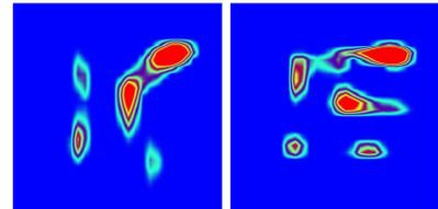
**Fig. 3:** Exp. NZ sand  $T_2$ - $T_2$  exchange plots,  $t_E = 50$  ms (right), 550 ms (left). Axes are logarithmic over the interval [3;300] ms.
