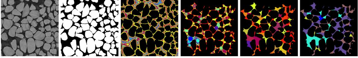
**Fig. 1:** Slices through a small sub-sample of NZ sand (1.7mm x 1.7mm) to illustrate from left to right: X-ray density map, segmented image, Euclidean distance map, covering radius map, and pore partitions. For the two pore partitions (right) colours are assigned by equivalent sphere radius reflecting volume and volume/surface ratio.
